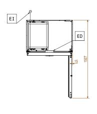
Electric Supply voltage: 220-240 V/1 ph/50 Hz Electrical power max: 0.45 kW Capacity: Number and type of grids (included): 5 - 530x700 **Key Information:** Net Volume: 510 It Door hinges: External dimensions, Width: 900 mm 700 mm External dimensions, Depth: External dimensions, Depth with 1527 mm Doors Open: 2040 mm
